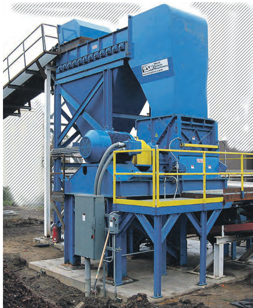
WSM's (West Salem Machinery) suggested their high capacity 5472 bark crusher with interchangeable tooling package after testing a sample of the eucalyptus bark at the testing facility.
