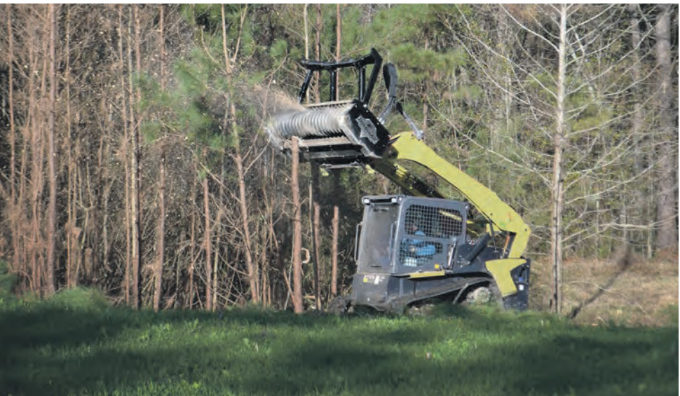
It uses a two-speed variable displacement piston motor, 41 hardened steel teeth and has a total attachment depth comparable to a loader bucket for easy operation and better visibility.
