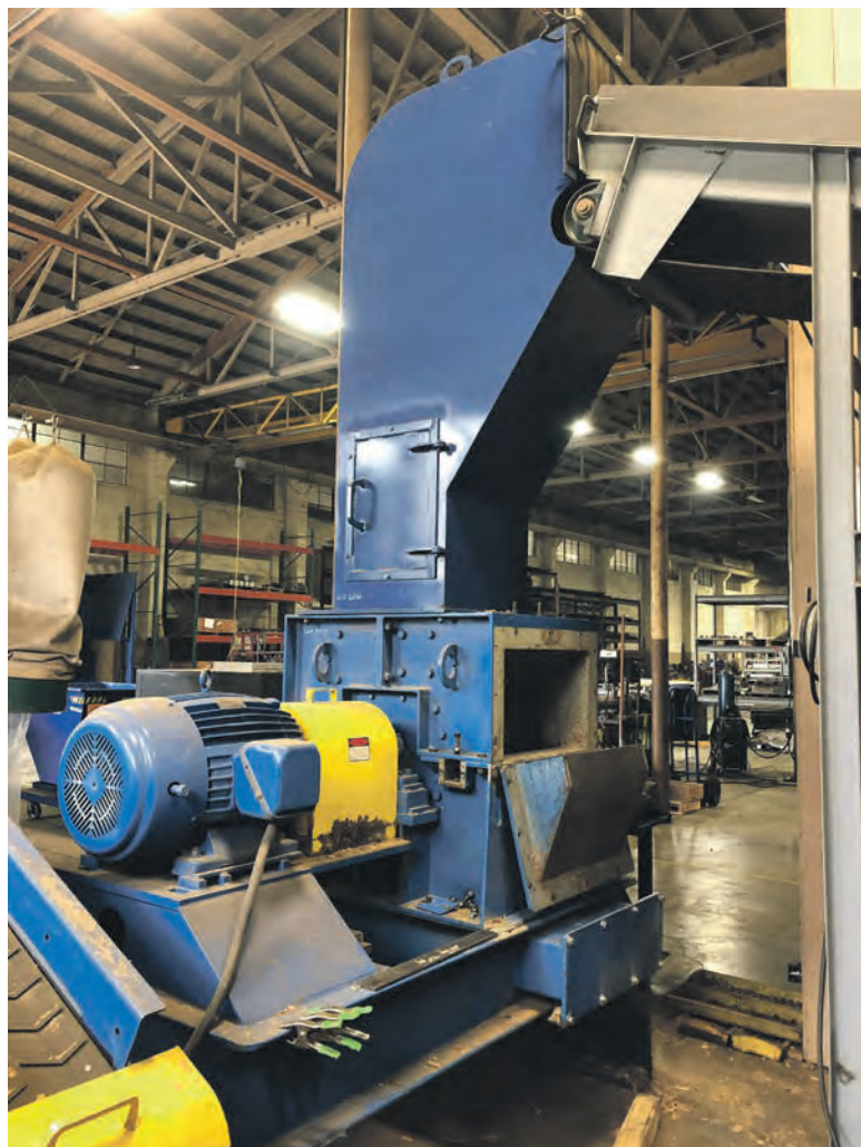
The test facility is equipped with a horizontal grinder, primary shredder, high-speed hammermill, full air discharge capabilities, disc screen, oscillating screen and screening equipment for sieve analysis.
