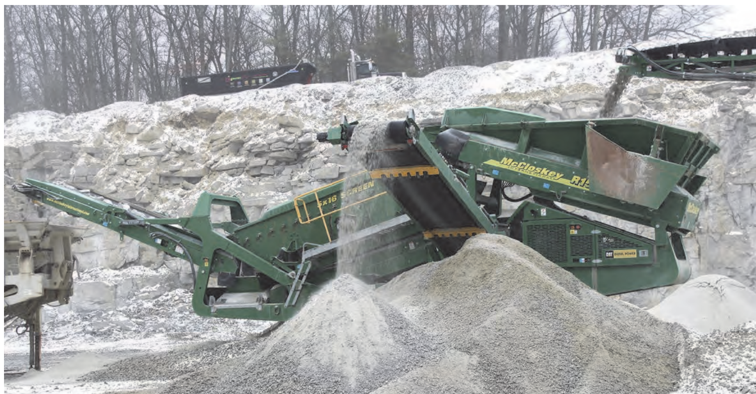
One of the three R155 screener scalpers producing one product, and feeding a jaw crusher over-size for further processing.
