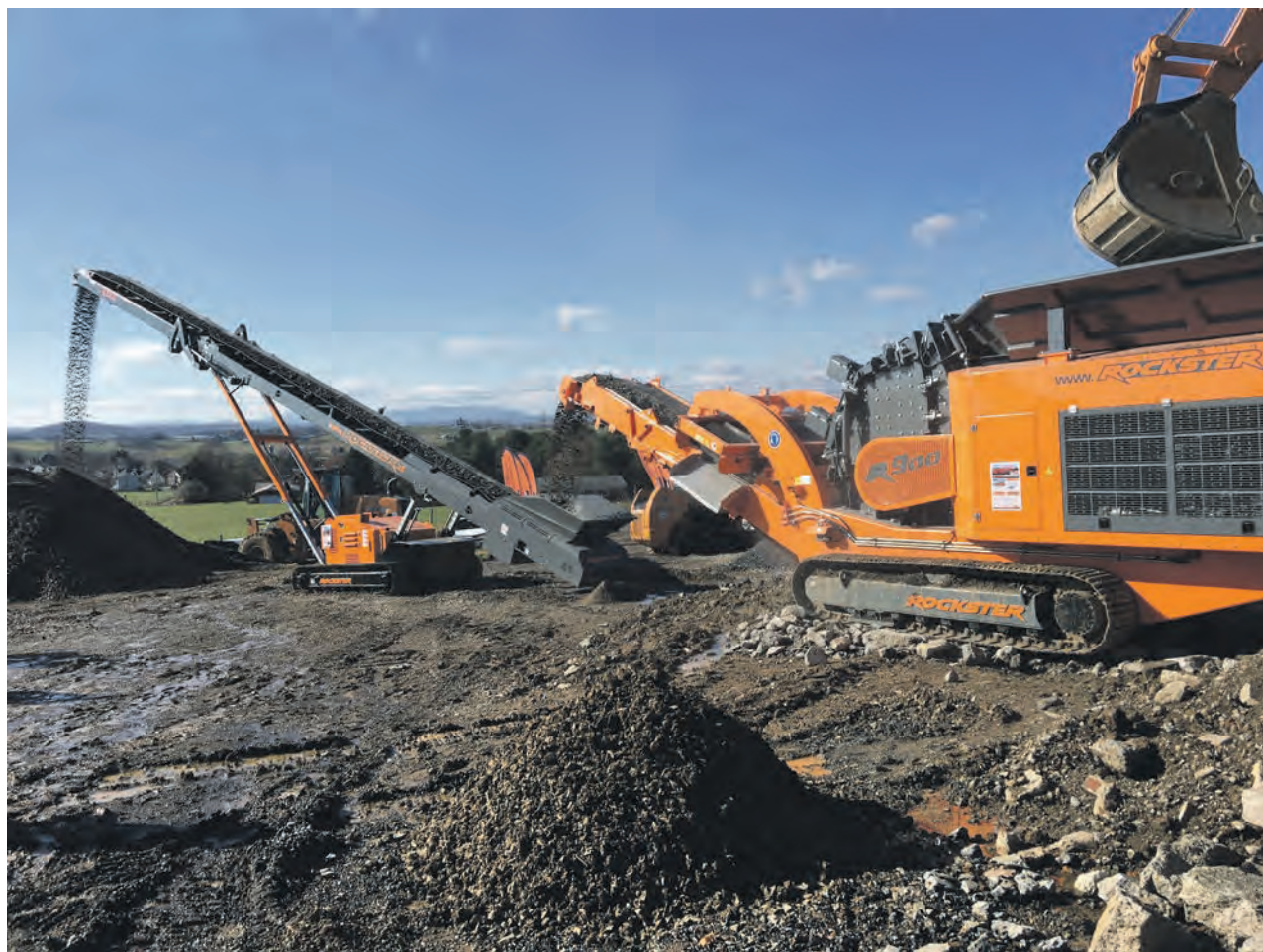
The impact crusher R900 with Duplex System together with the stacker RST18 at the processing of concrete.
