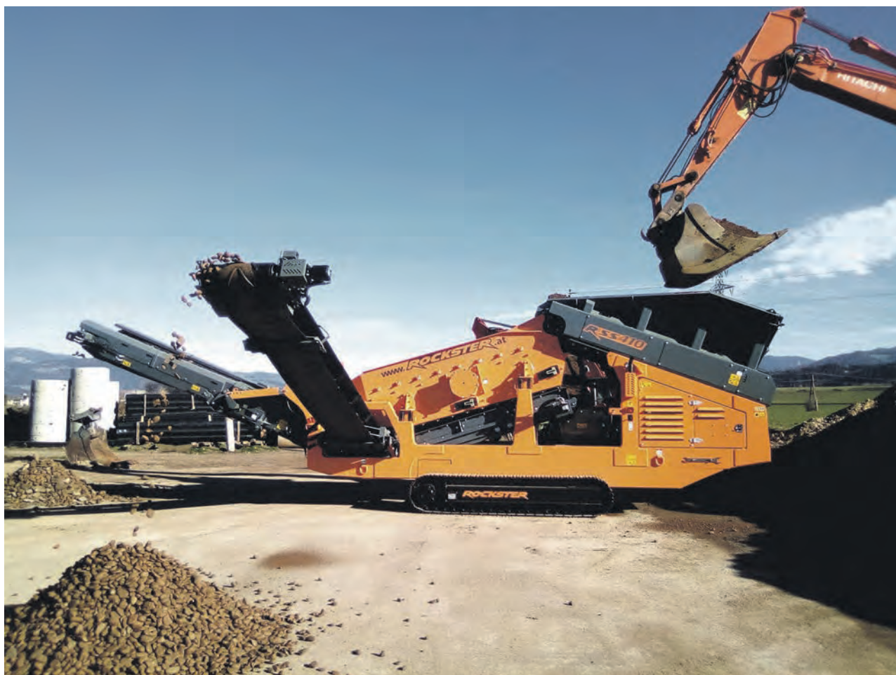
The ROCKSTER RSS410 2-deck scalping screen at the separation of topsoil.
