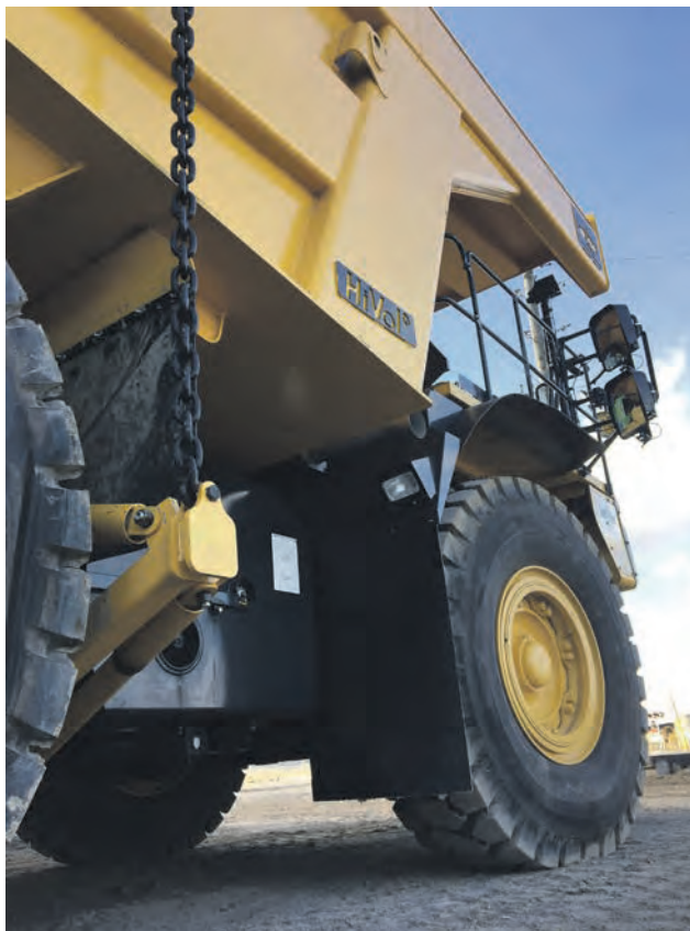
Philippi-Hagenbuch's newest Autogate® Tailgate innovation is designed with a traditional outrigger that bolts to the undercarriage of the off-highway truck, allowing operators to retain Komatsu's original OEM truck frame warranty.
