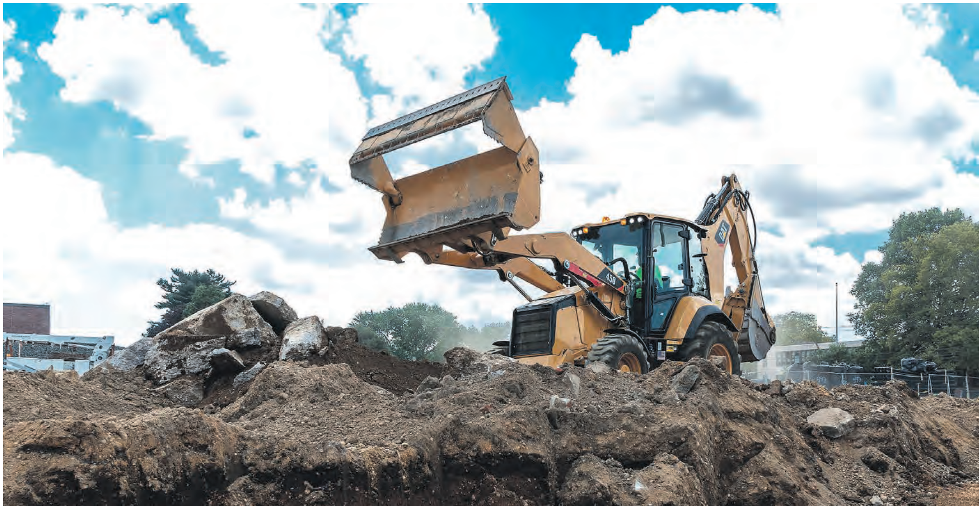
The powertrains for both models are anchored by the Cat C4.4 ACERT™ engine, which meets stringent Tier 4 Final emissions standards using a service-free SCR solution for improved operating efficiency.
