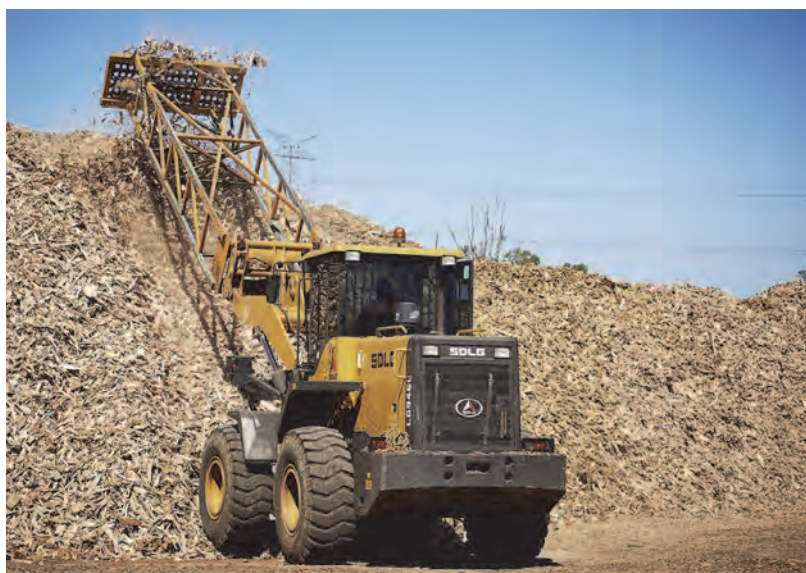
ALG946L uses a specialized attachment to push pallet offcuts up and onto the stockpile.
