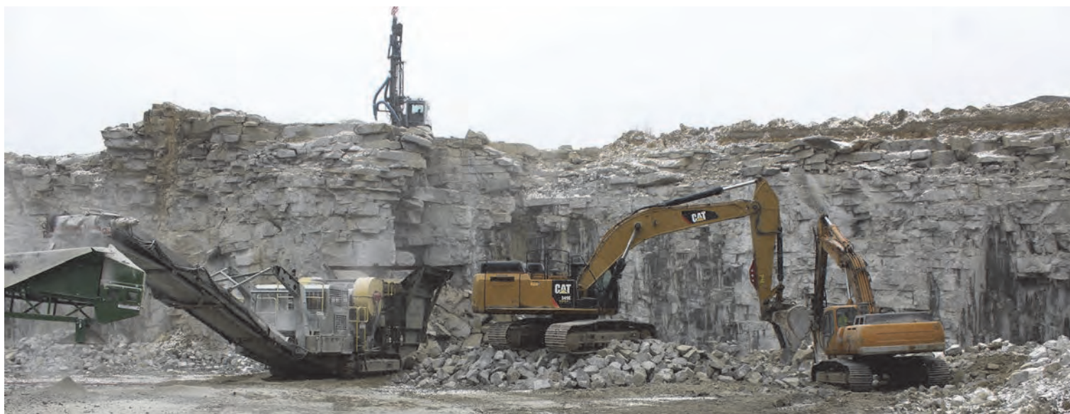
One of W.J. Graves' quarry sites with primary crusher, drill rig, excavators and a stockpiling conveyor.
