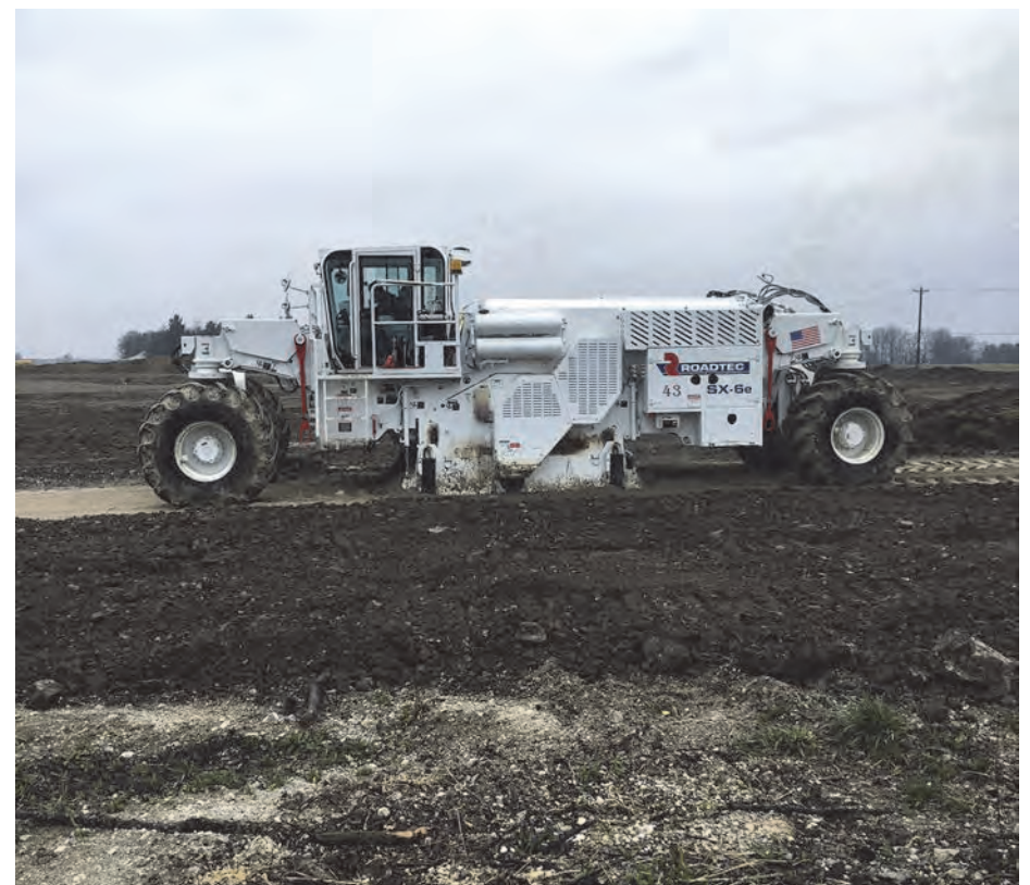
The machine is capable of cutting up to 20 inches (508mm) deep and 100 inches (2,540mm) wide.
