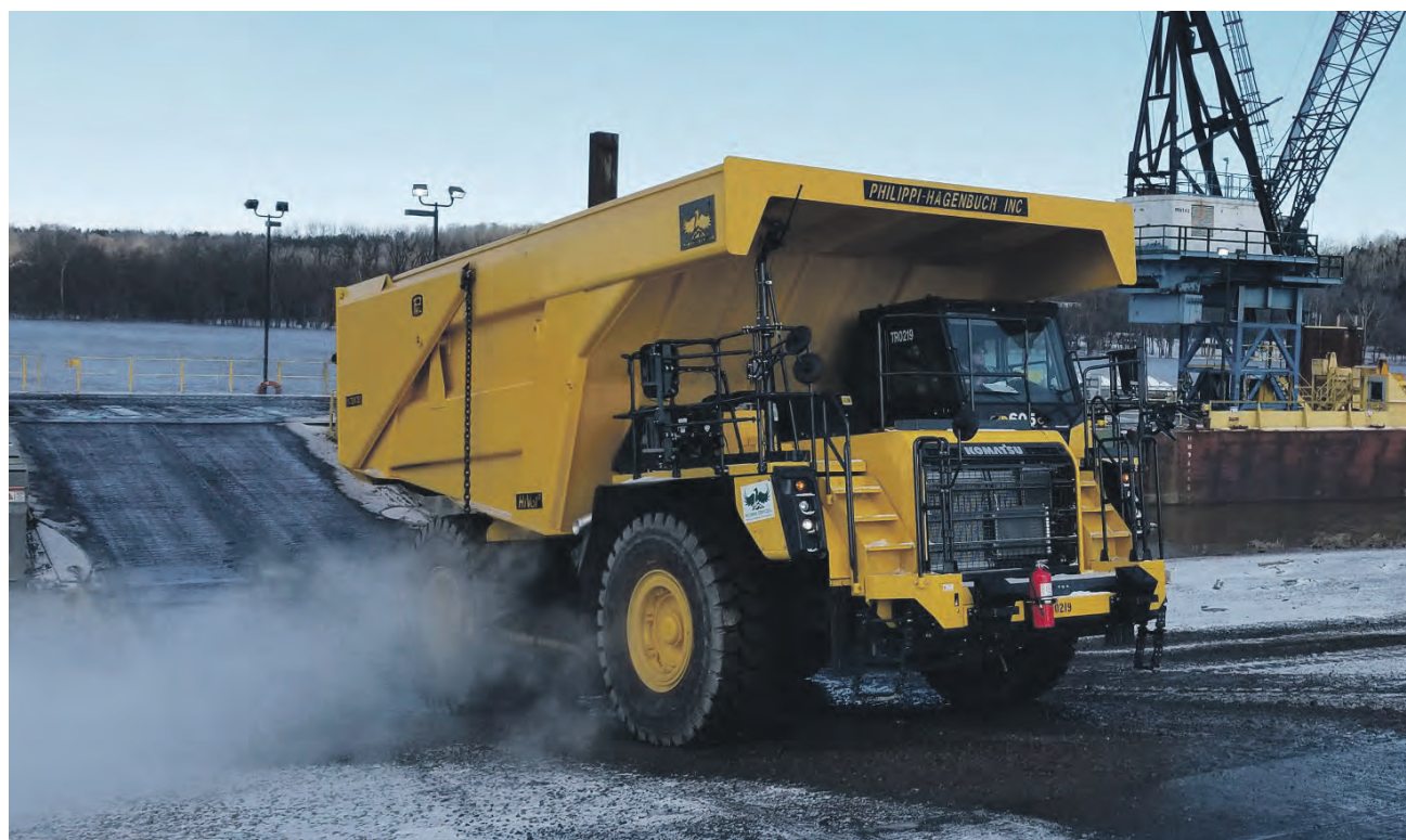
Philippi-Hagenbuch Inc. unveils a new version of their Autogate® Tailgate specially designed for Komatsu rigid frame trucks.
