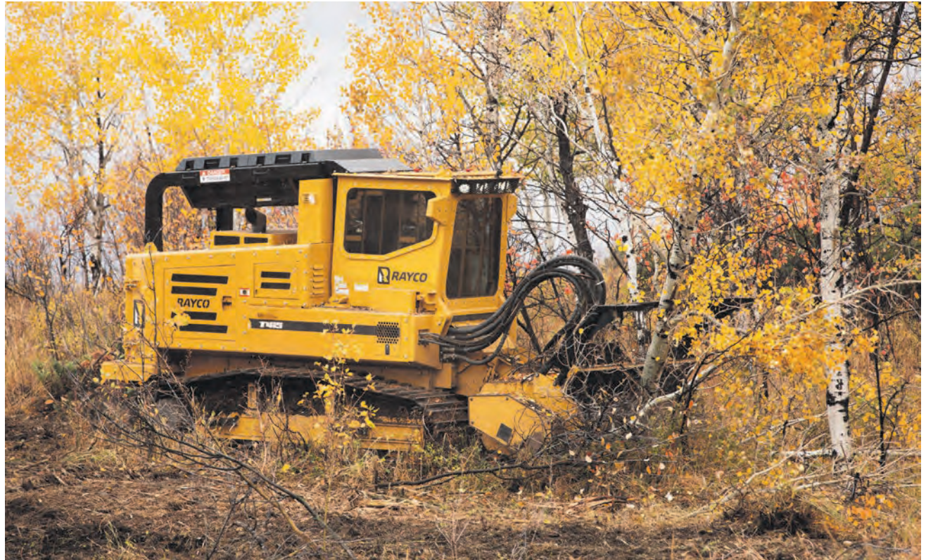
For mowing/mulching applications, the Predator mulcher head has a 91.25-inch cutting width.
