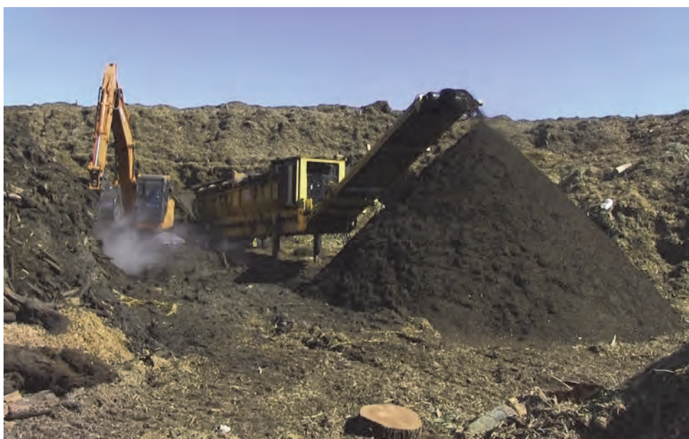
A Vermeer trommel plays an important role in turning waste wood into compost for GPO.
