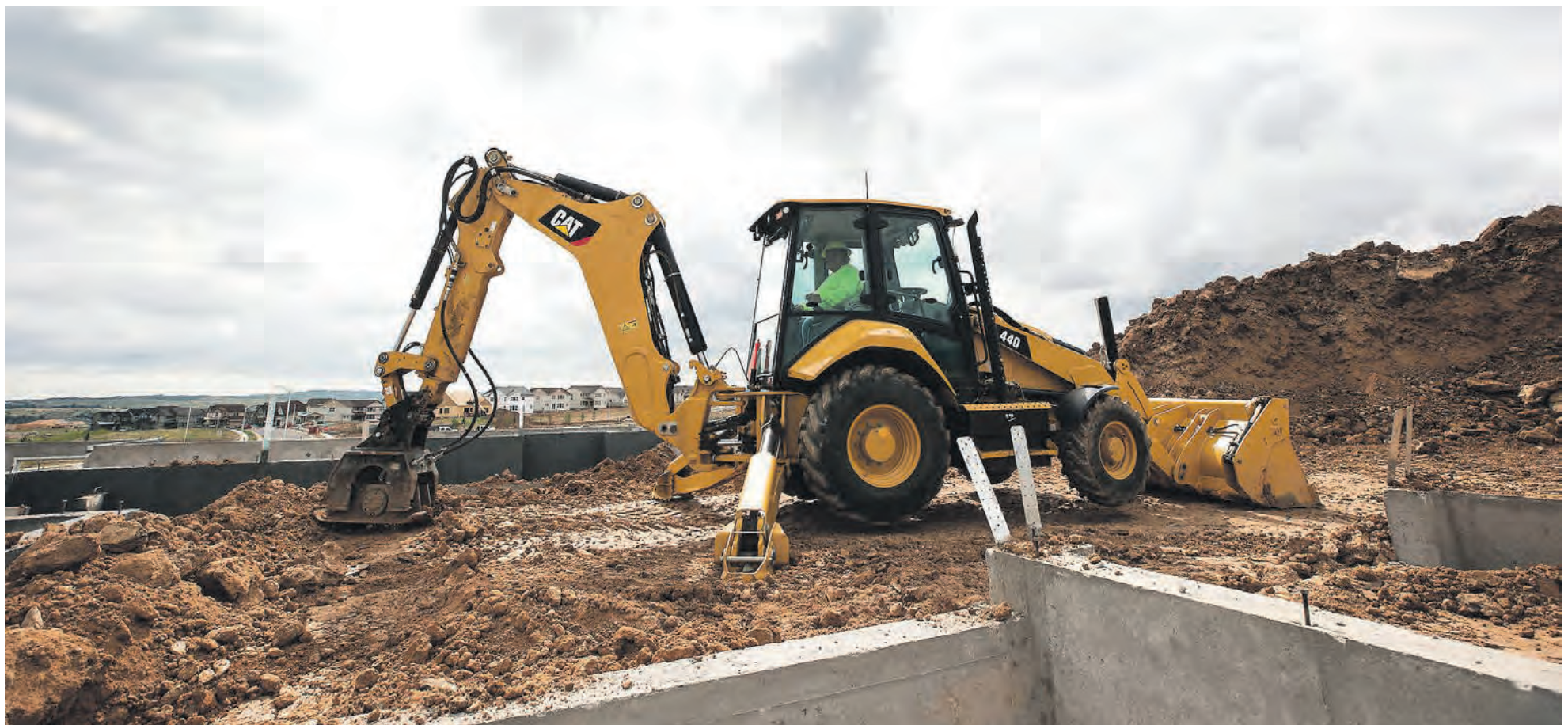
These new backhoe loaders feature adjustable auxiliary hydraulic flow to the work tool to efficiently operate powered attachments.
