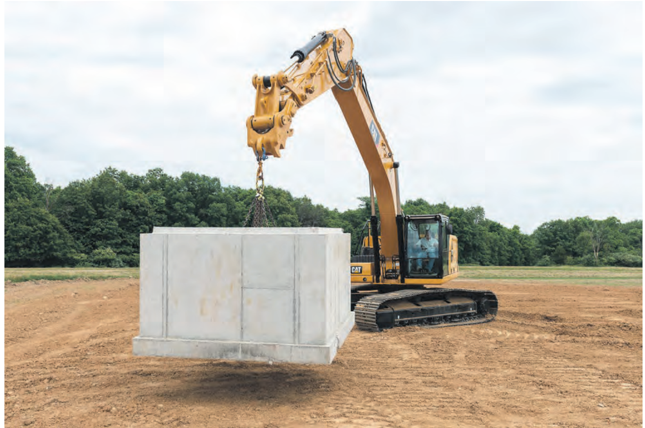
The new Lift Assist feature helps the operator safely pick up heavy objects without tipping.
