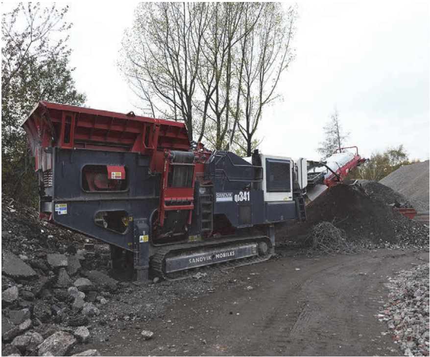
SJ Walchester’s recently acquired QJ341 tracked jaw crusher from Sandvik has impressed all at the company with its reliability, effectiveness and ability to crush asphalt and tarmac even in warm weather.
