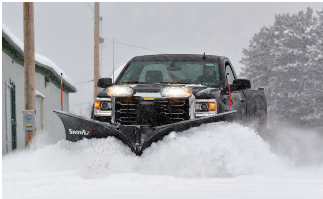
Whether the plow is in scoop, angle or straight blade position, an independent trip edge protects the plow, truck and operator when encountering obstacles.
