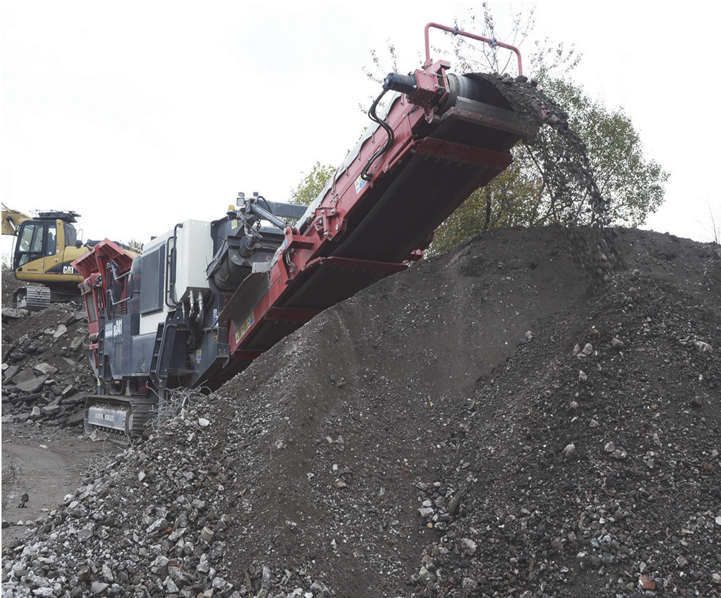
QJ341 is the only jaw crusher Walchester has experienced which will process asphalt and tarmac without problems.
