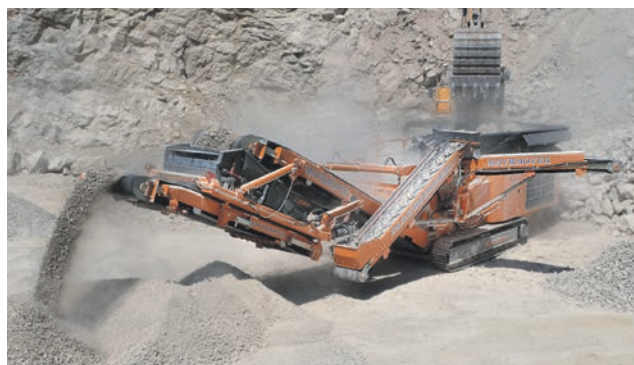
Using the return belt as a stockpiling belt produces a further final fraction.
