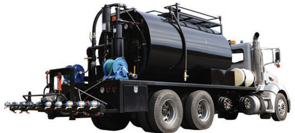
Individual nozzles can also be controlled from the truck cab, giving contractors the flexibility to adjust the spray area as needed.
