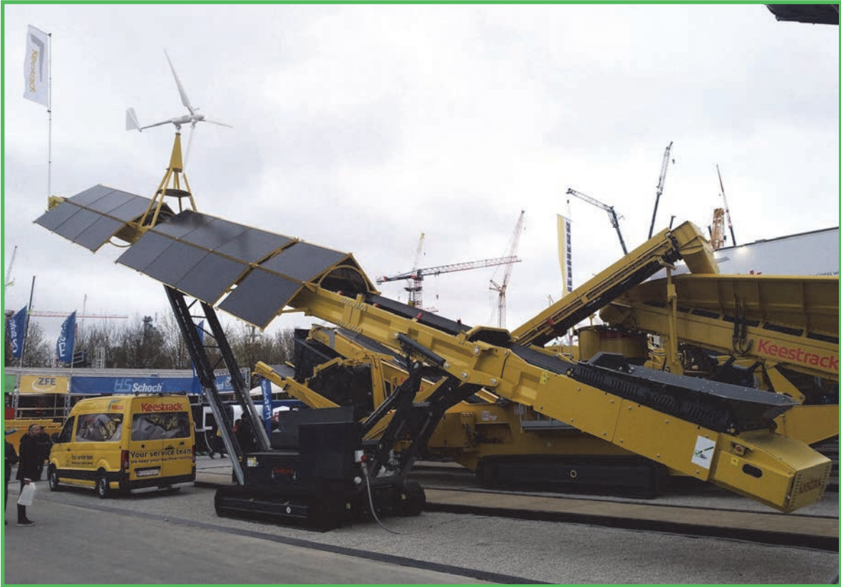
The S5e Solar is possibly the first directly solar-powered mobile processing plant worldwide.
