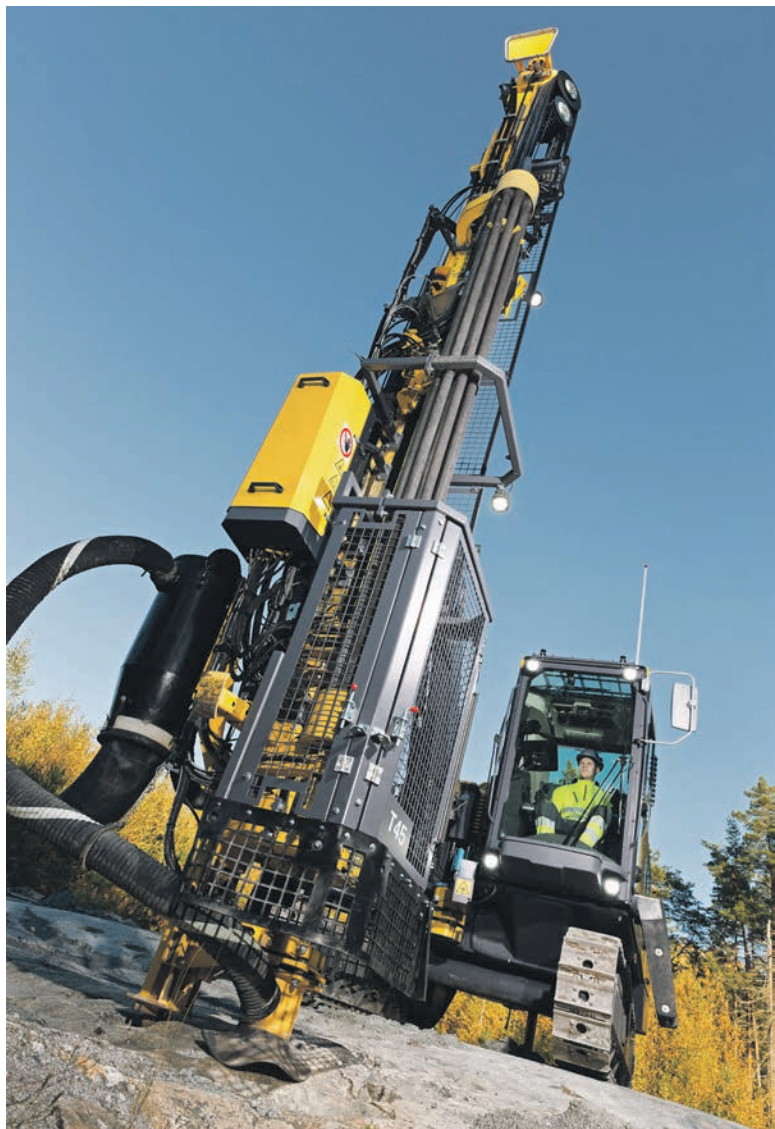
Epiroc's fuel-efficient SmartROC T45 comes with its own site-navigation system.
