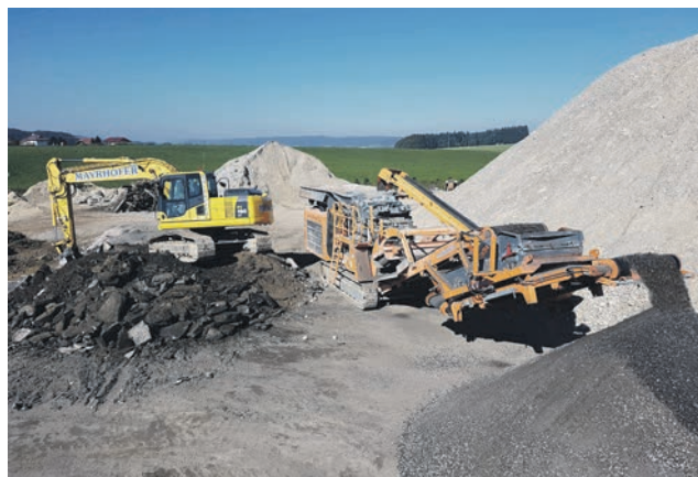
Asphalt recycling to a final grain size of 0 - 32 mm (0 - 1.26 in) at the recycling area at Mayrhofer's headquarters in Neumarkt.
