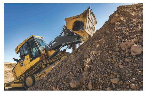
The 655K and 755K (shown) boast hydrostatic transmissions, a feature John Deere pioneered in crawlers in North America in 1976.
