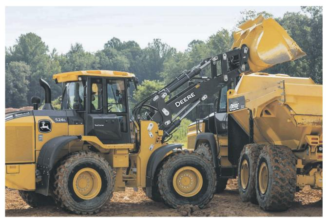
Additional bucket options include enhanced production buckets with integrated spill guards, profiled side cutters and greater rollback, improving bucket fill and material retention.
