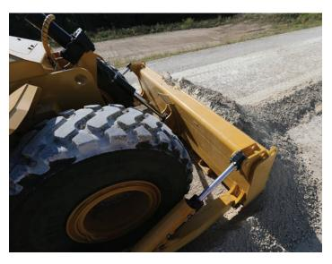
The 2.84-m<sup>3</sup> (3.72yd<sup>3</sup>) straight blade delivers high production dozing on stockpile material and general earthmoving projects.
