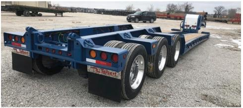
The Talbert 60CC/55SA-LD is a hydraulic detachable gooseneck trailer featuring a nonground bearing hydraulic gooseneck design.
