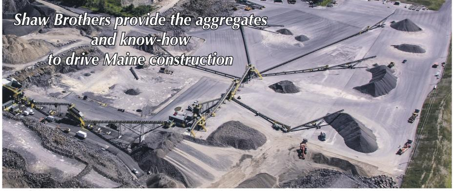
Bird's eye view of the new crushing plant, a 37 acre paved site with extensive conveyor systems reducing emissions from trucking and loading equipment.
