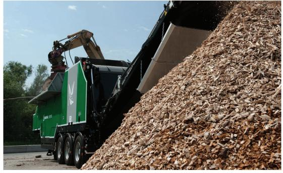
Simply exchanging the free swinging tools for fixed tools converts the Axtor into a powerful chipping machine for logs.
