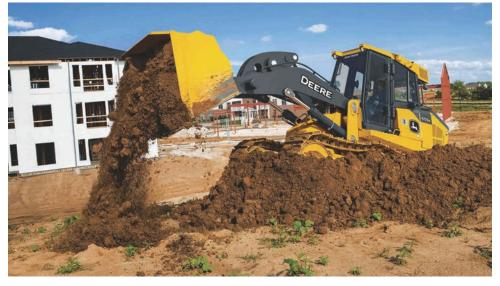
Both the 655K (shown) and 755K are equipped with Eco Mode, yielding up to 20 percent less fuel consumption with no loss in productivity.
