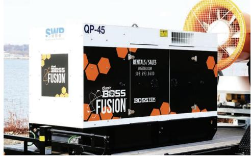
The system's gen set is powered by a heavy-duty 4-cycle diesel engine.
