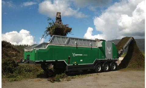
solid lowers the A fuel with a coarse structure can be generated from woody green waste, clean waste sulphur dioxide content of the wood and forest wood residue by shredding.
