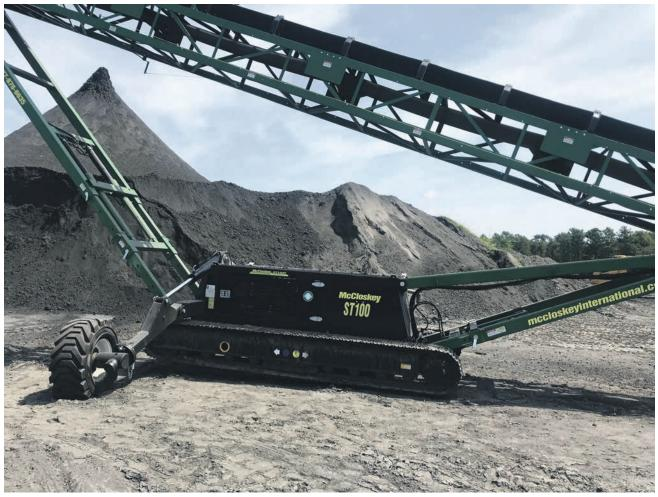
The lift axle option allows switching from track mode to radial in seconds
