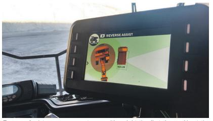
Reverse Assist ensures operators position right the first time, without the need for shovel-bucket support.
