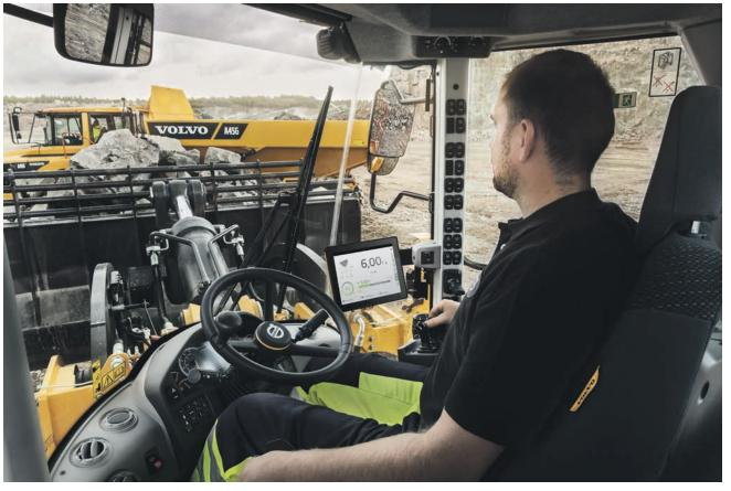
Dig Assist Start and Load Assist provide real-time guidance for operators to enhance performance, productivity and safety. Photo courtesy of Volvo CE
