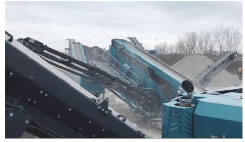
The Powerscreen impact crusher and screener are vital components of the recycling operation.
