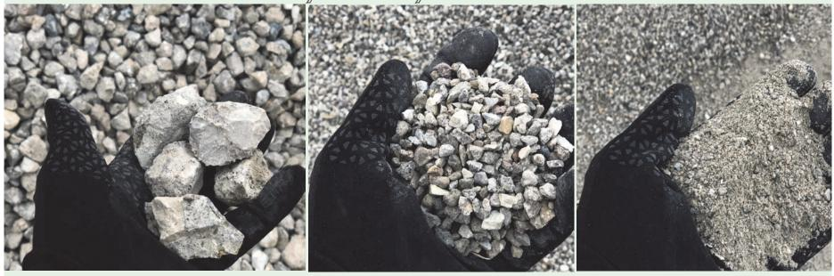
Clean aggregate is produced at site from material that would have traditionally been seen as waste: CA1/CA16 and FA6.
