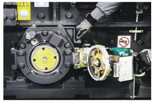
A new rotor position and locking device, new hammer locking wedges for quicker removal and fitting and a new wedge removal tool provide safer installation and removal.
