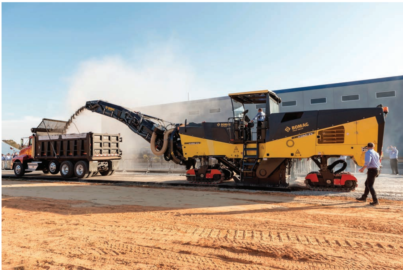
The outer conveyor swivels 60° left or right of center and discharges material at a height of 16.4 ft (5 m).
