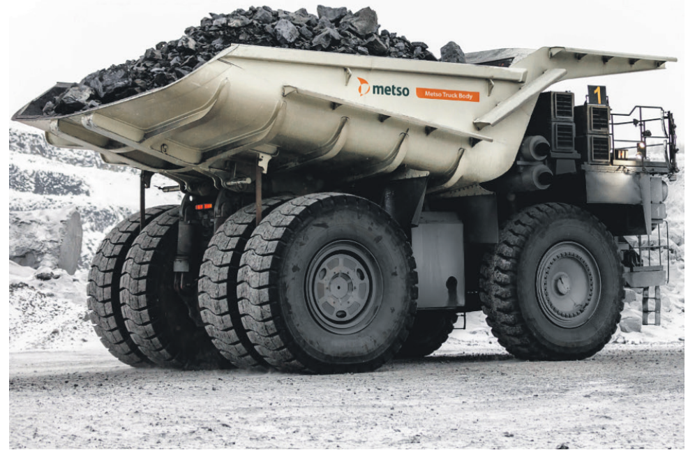
The Metso truck body is a groundbreaking innovation that combines the benefits of rubber and high structural strength steel.
