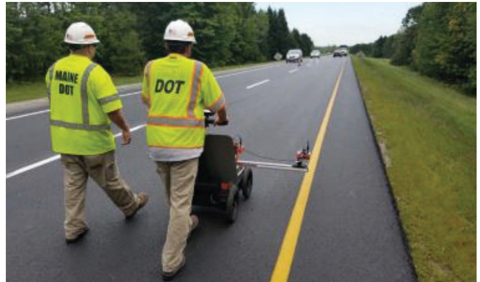
According to SHRP2 studies, GPR can be used to measure uniformity and potential defect areas in asphalt pavements during construction.
