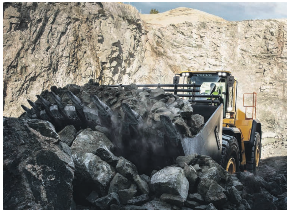
The new tooth system helps to distribute stress while working.
