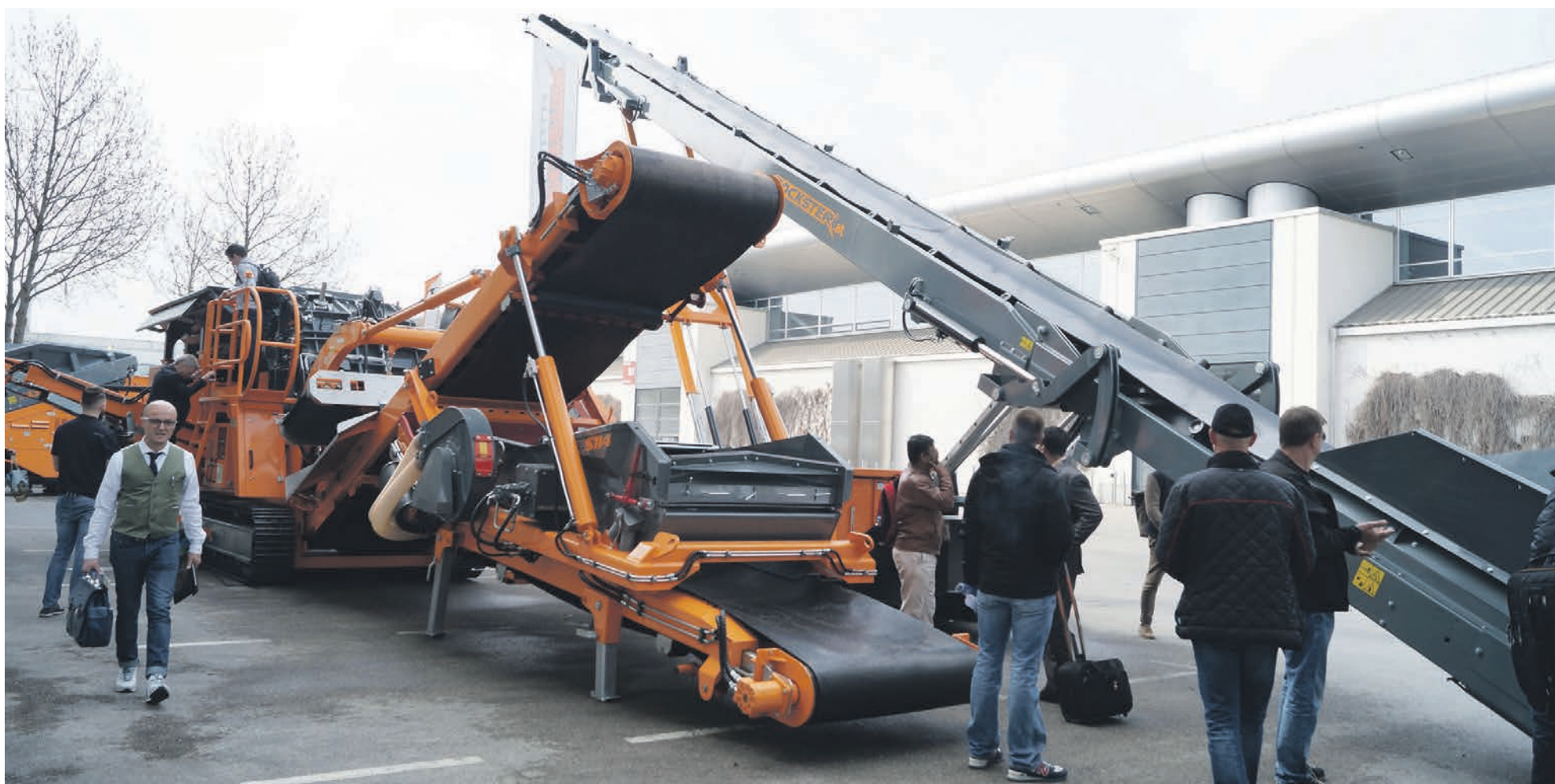
At Rockster's outdoor area, visitors could take a closer look at the air blower or the hydraulically foldable screening system of the impactor R1100DS.
