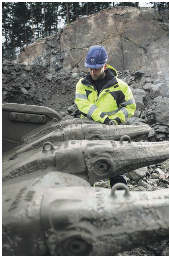
The teeth and adaptors are specifically matched to the specification, size and model of machine.
