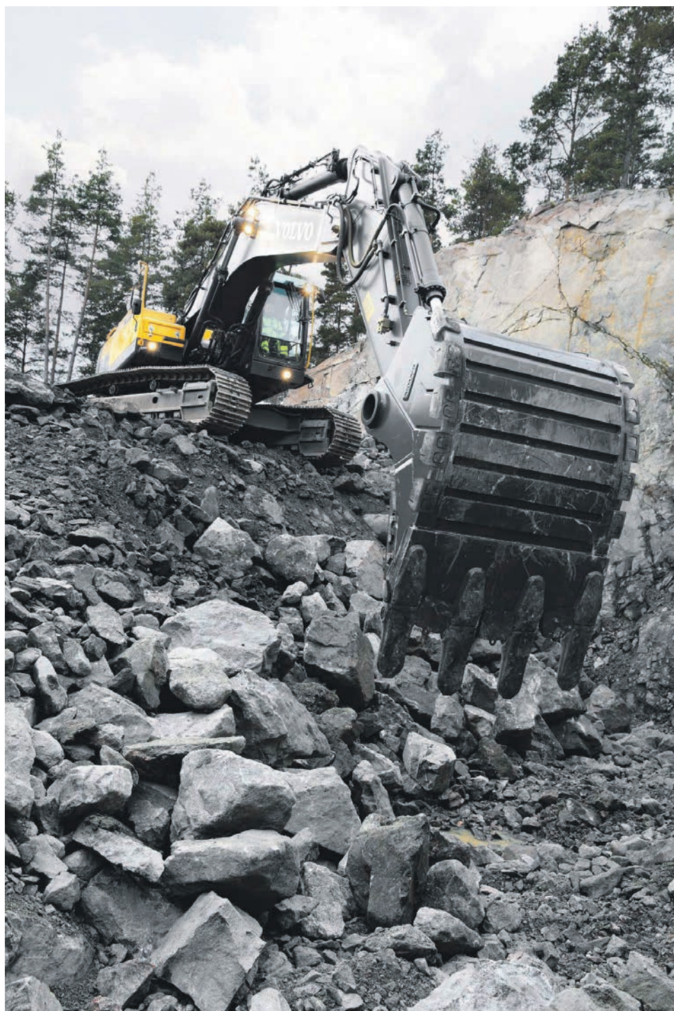
Volvo's new tooth systems has a longer life and higher penetration.
