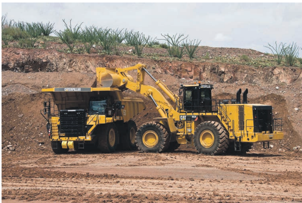
Rated payload for the new 777G is 98.4 tons (89.4 MT), with a standard-body volume (SAE 2:1) of 83.8 cubic yards (64.1 m 3 ).
