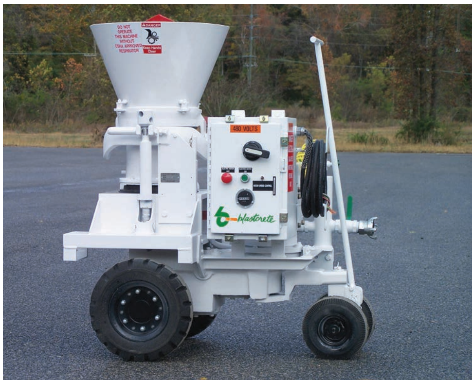
Blastcrete Equipment's Piccola guniting machine is a simple solution for gunning applications up to 6 cubic yards per hour.
