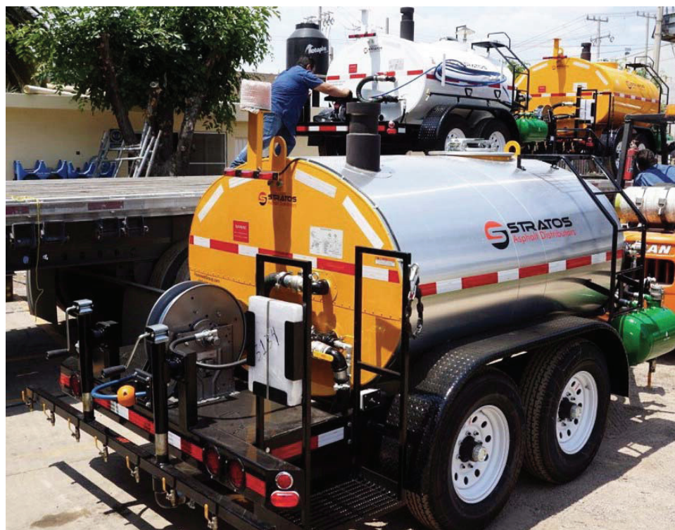
PavementGroup also manufactures Stratos asphalt distributor trailers — in capacities from 400 - 2,000 gallons — with a worldwide customer base. Pictured is a 1,000 gallon example.
