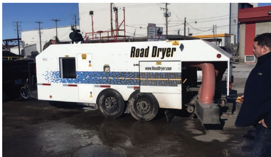
Road Dryer's trailer and truck-mounted pavement drying units quickly dry asphalt and concrete pavement, allowing crews to pave or apply surface treatments or striping after just one pass.
