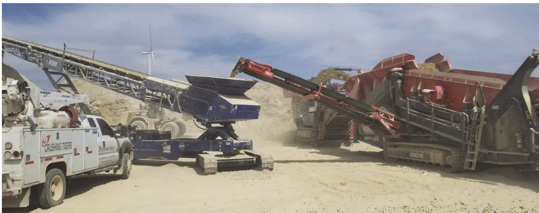
Product from the scalper being fed directly into a tracked conveyor.
