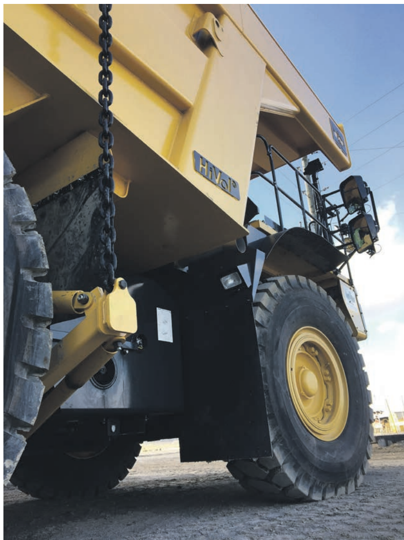
This new design does not require any welding to the frame, allowing operators to retain Komatsu's original OEM truck frame warranty.
