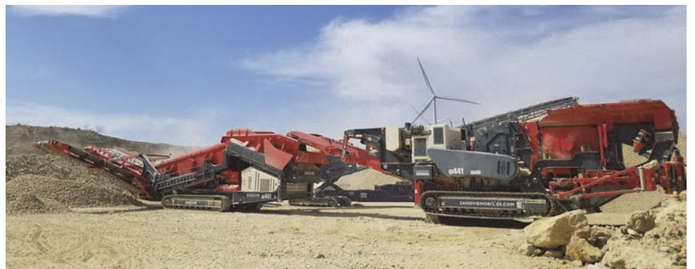
Depending on the specific requirements of the customer and the set-up of the crushing and screening train, production in the range of between 200 – 500 tons per hour is readily achievable.
