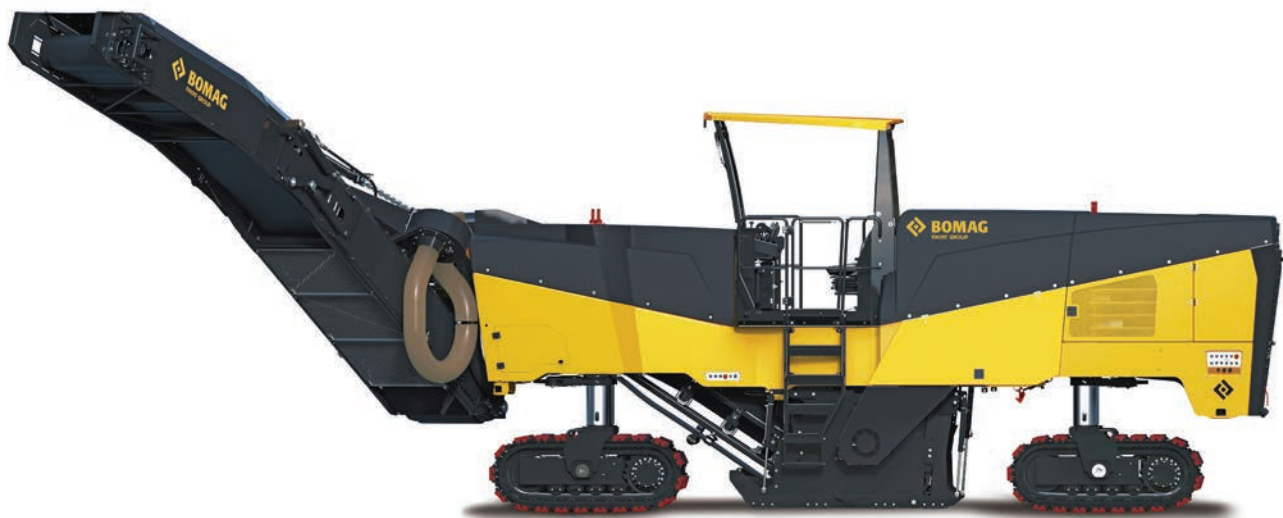
With its powerful 760.3-hp (567-kW) diesel engine, the BOMAG BM 2200/75 delivers high-performance milling of half-lane widths reaching 86.6 in (2,200 mm) at precise milling depths of up to 13.8 in (350 mm).
