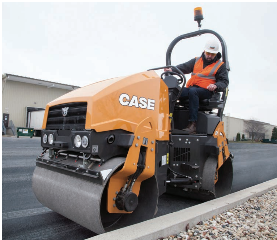
The drums can be offset to further improve accessibility, and to improve performance during turns.
