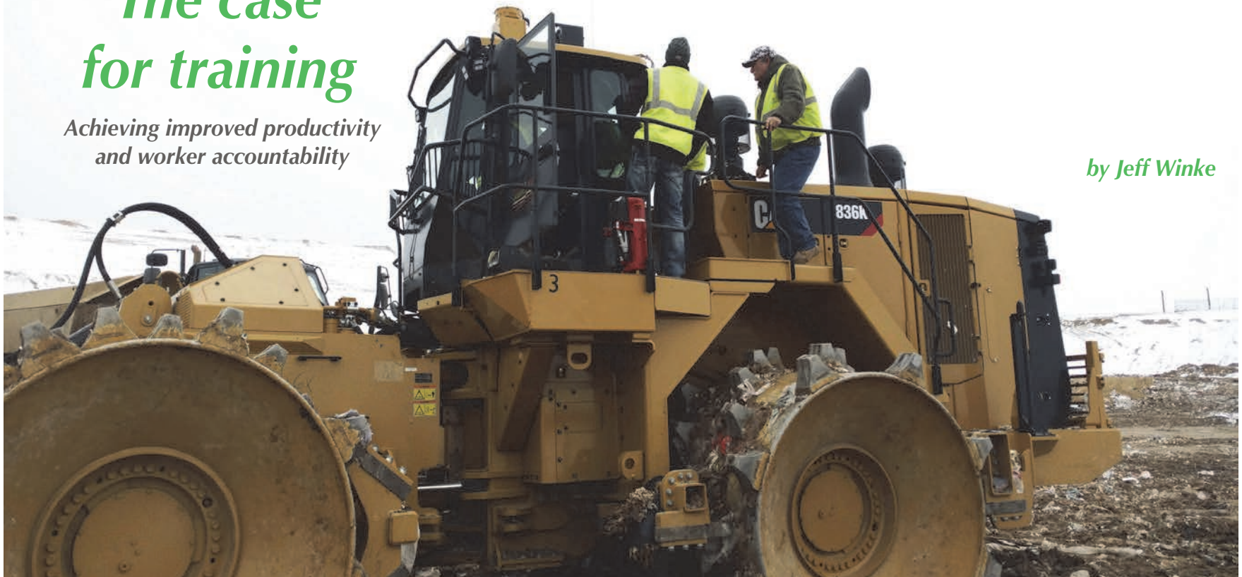
Trans-Jordan uses two Cat 836K Landfill Compactors working together, equipped with the JohnnyBall 3D level and slope measuring system..
