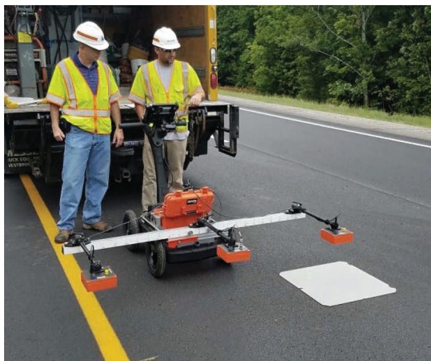
PaveScan RDM set up with three 2-GHz sensors mounted on a portable push cart.
