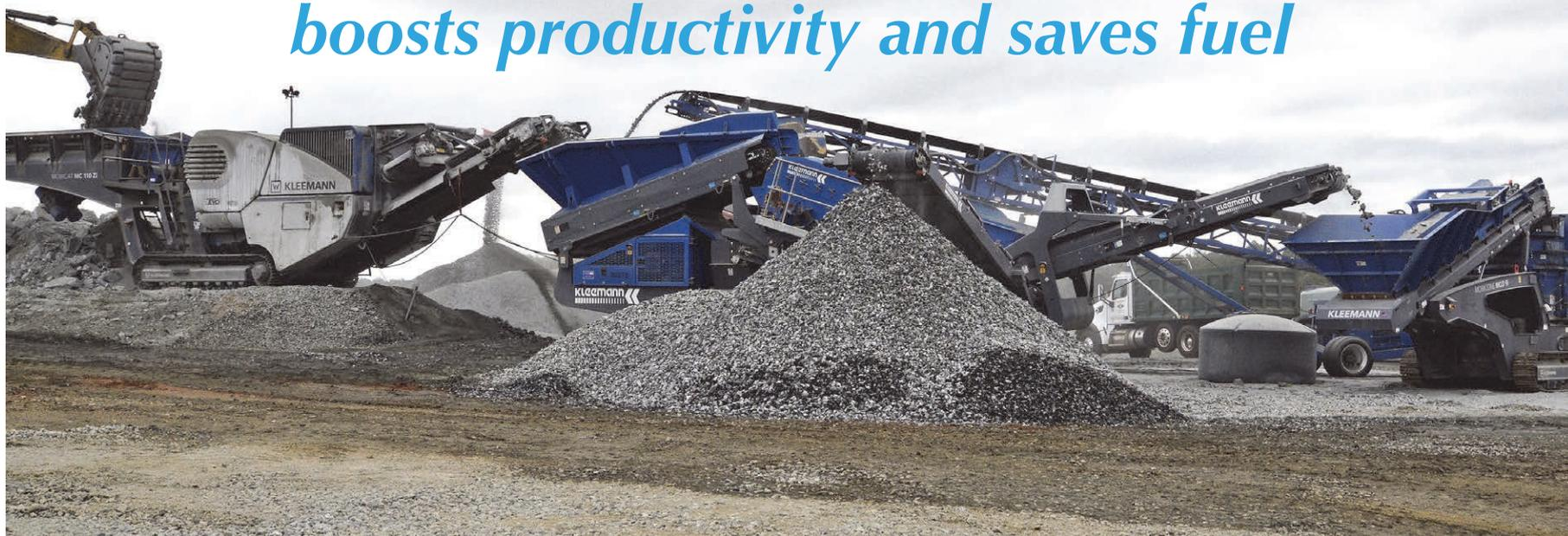
Kleemann Mobicat MC 110 Zi EVO primary jaw crusher, Mobiscreen MS 15 Z screen, and Mobicone MCO 9i EVO secondary cone crusher work together in Interlinked mode.
