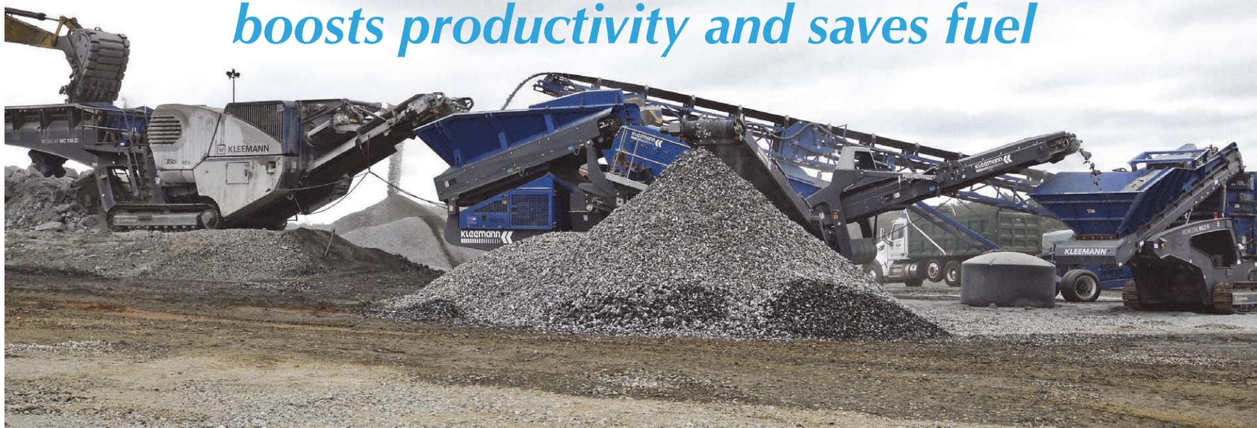
Kleemann Mobicat MC 110 Zi EVO primary jaw crusher, Mobiscreen MS 15 Z screen, and Mobicone MCO 9i EVO secondary cone crusher work together in Interlinked mode.
