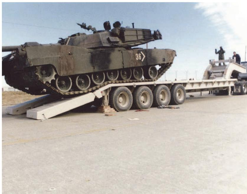
*The Talbert trailer allowed for safe loading and hauling of the some of the heaviest and unique equipment known at the time.*
