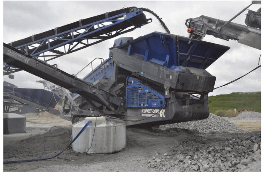
Jaw (right conveyor) and cone crusher (left) send aggregate to the Kleemann Mobicat MS 15 Z for further classification.
