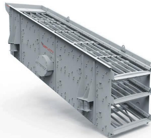
The SI screens are built with a robust drive mechanism and oversized bearings to handle large tonnages and a wide variety of applications.
