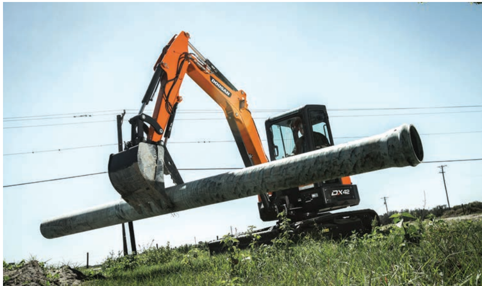
Doosan DX42-5 is a conventional tail swing mini excavator in the 4- to 5-ton class. Photos courtesy of Doosan
