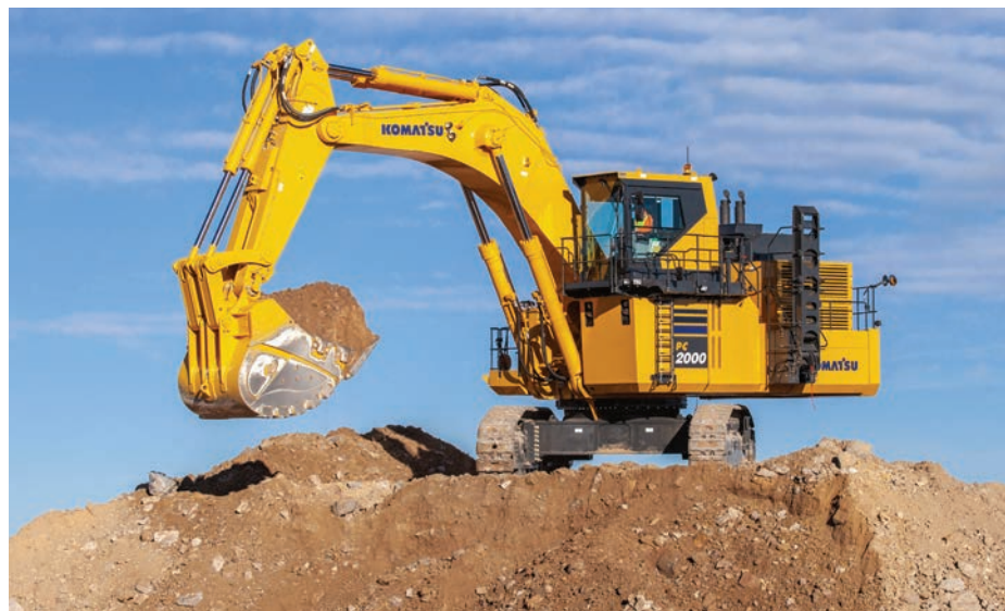
Increased engine power and new engine pump control logic give the PC2000-11 faster cycle times.
