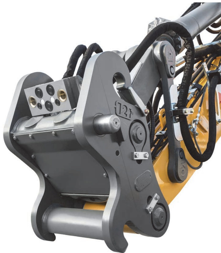
Likufix system is owned by Liebherr and is strong in German-speaking markets, with a corresponding linkage to operators of Liebherr excavators.
