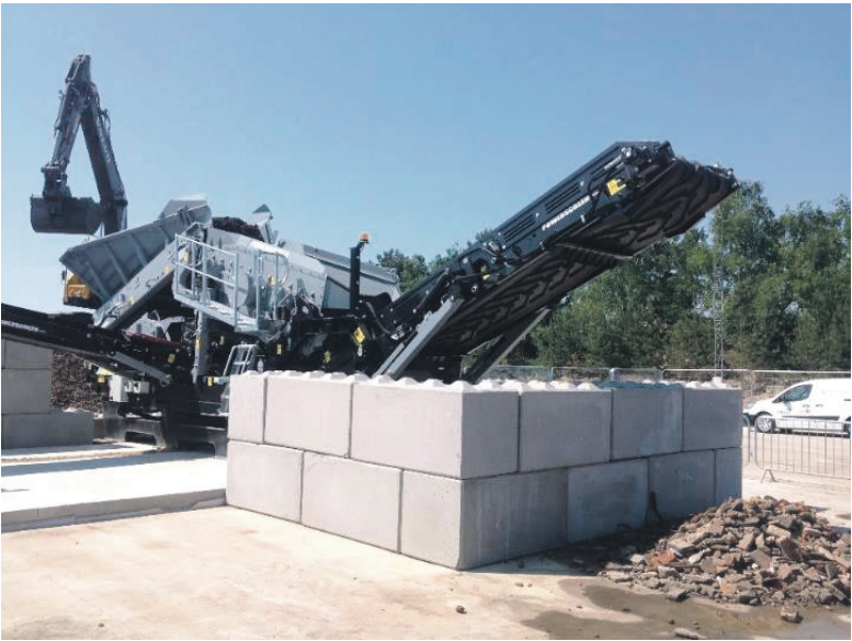
This unit removes excess oversize before passing the bulk of material to the subsequent washing equipment.
