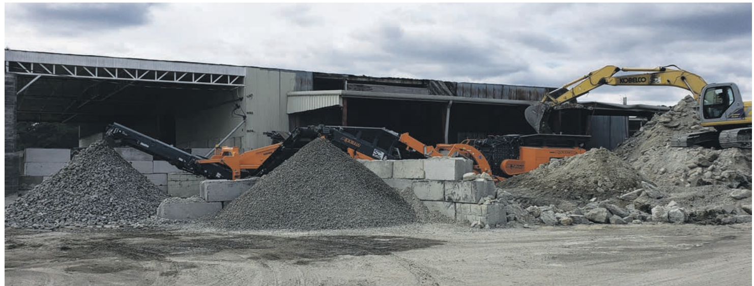
At the new South Carolina Recycling Center in Myrtle Beach, Michael Morais and his team crush and screen concrete for an immediate re-use in the Titan Enterprises' road construction projects.
