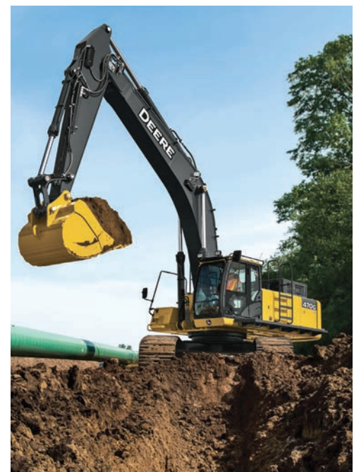
The integrated grade guidance system provides the operator with the bucket's location in relation to a 2-D reference or 3-D design surface. Photo courtesy of John Deere
