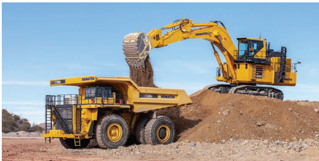
The PC2000-11 is designed to load 70- to 200-ton rigid frame haul trucks.
