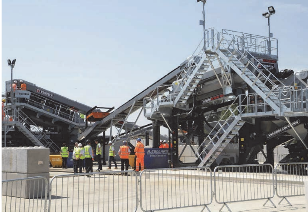
Terex Washing Systems recycling processes transform construction and civil engineering wastes into clean, homogenous recycled products.
