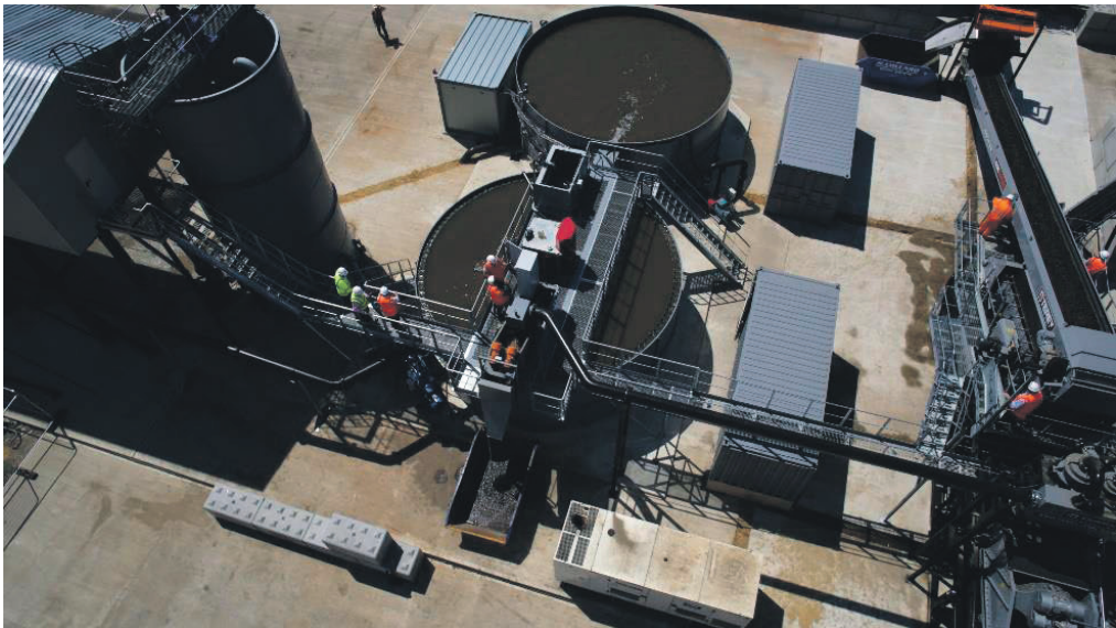
This thickener and filter press combination recycles 90% of the water used in the plant.
