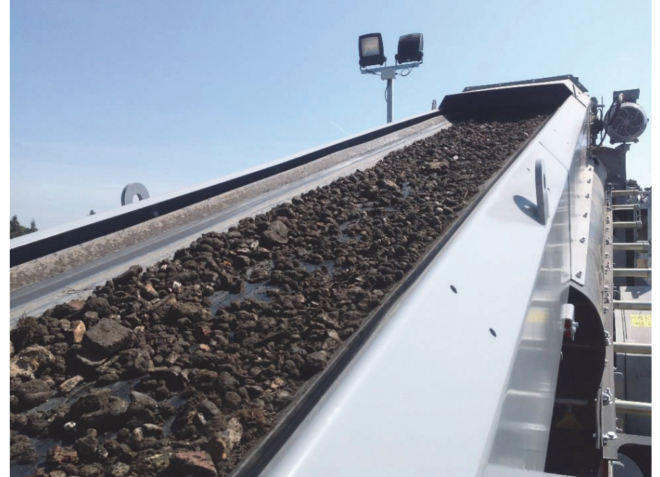
The process starts with a Warrior™ 1400 heavy duty scalping unit particularly suited to claggy and clay contaminated/high soil content feeds.
