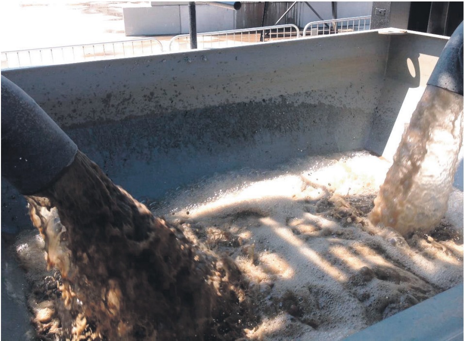
Sand and water from the AggreSand screen together with return water.
