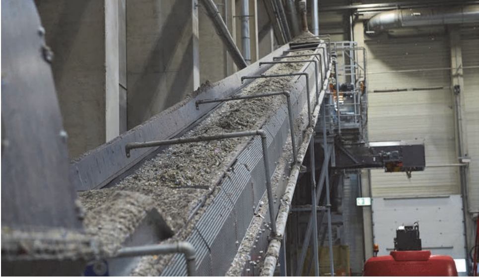
After shredding, the fuel particles are transported to the processing unit.
