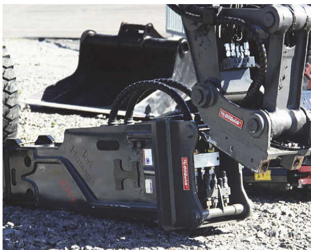
OilQuick quick couplers have been developed to enable the quick and safe switching of hydraulic attachments directly from the cab.
