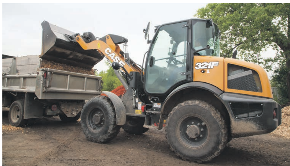
The new electro-hydraulic controls also offer automated bucket metering functionality. Photos courtesy of CASE CE
