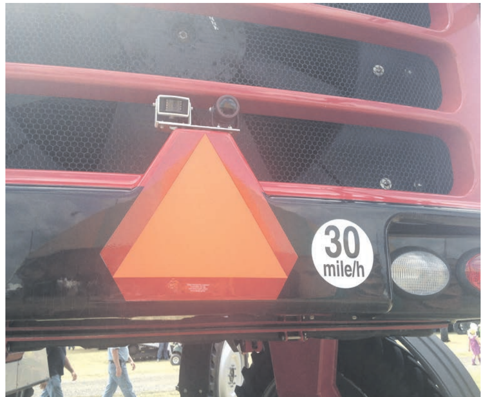
A speed identification symbol (SIS) is newly required by New York State law for equipment that moves between 25 and 40 mph.
