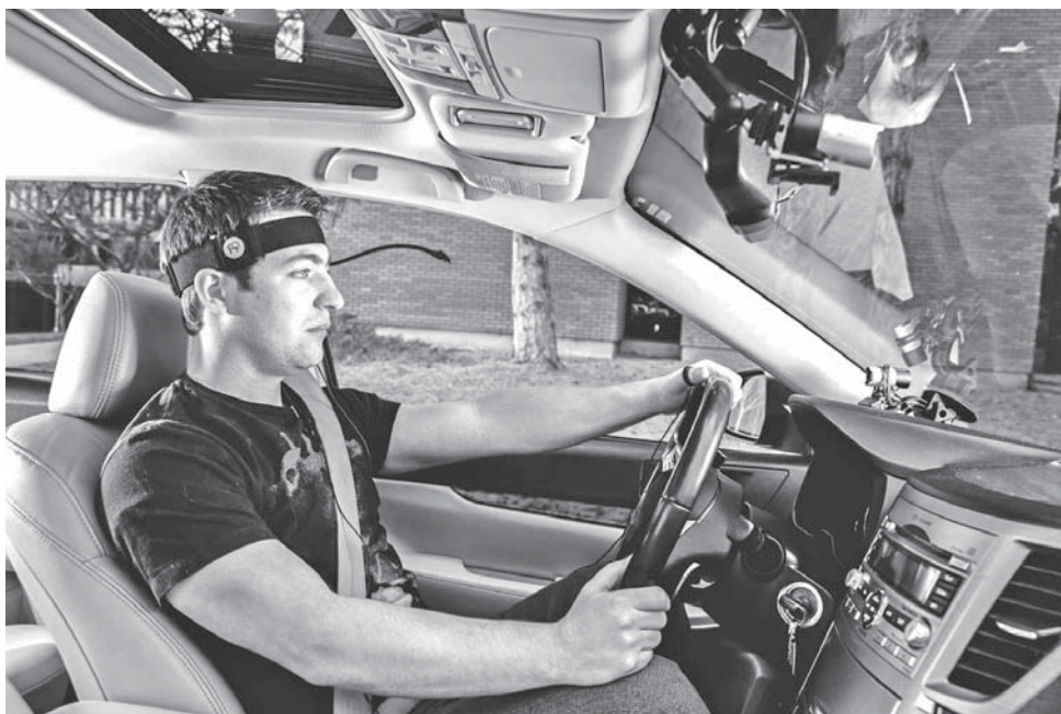
The AAA Foundation for Traffic Safety sponsored two University of Utah studies on how in-vehicle, voice-controlled infotainment systems distract drivers more than is commonly believed. Here, a study participant drives and makes voice commands while a camera and other instruments measure his level of distraction.
