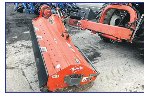
Kuhn TB211 Offset Flail Mower - PTO Driven, 6'8" Working Width, 3 Point Hitch $7,975
