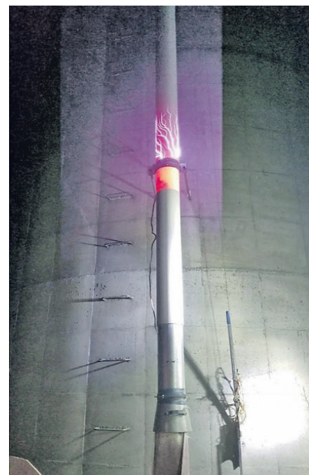
Plastic (PVC) pipe is not recommended for crops at less than 50% moisture due to the hazards of static electricity. Thank you Pitzke Farms Inc for permission to share this picture.
