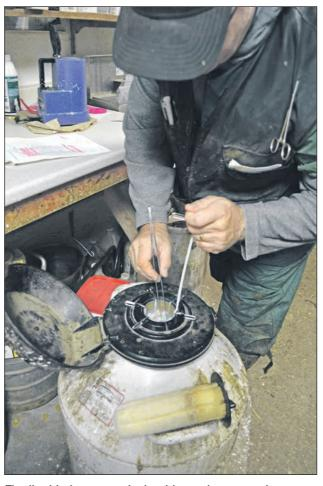
The liquid nitrogen tank should remain open only as long as it takes to remove the correct straws.
